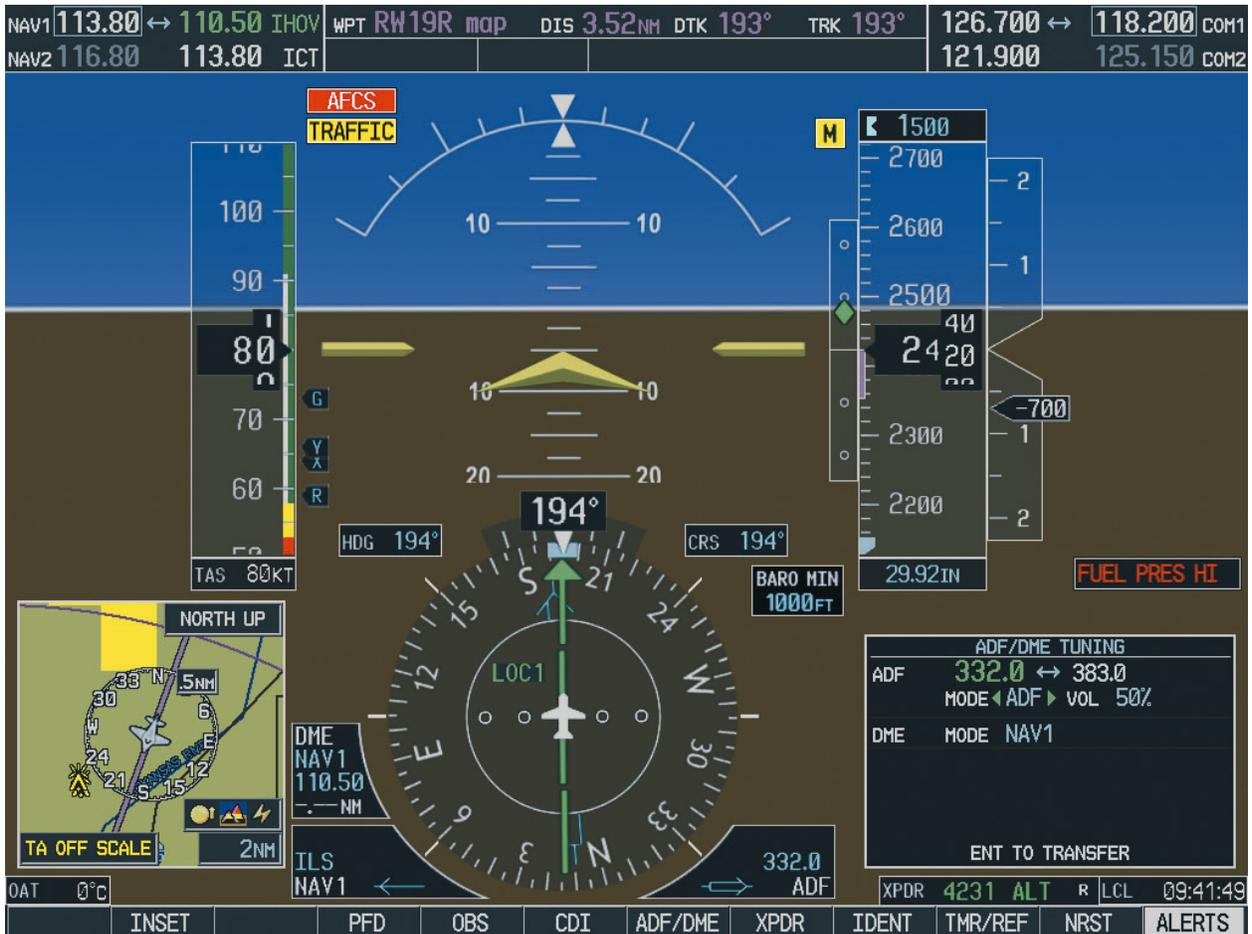
Figure 2 GDU 1040 Primary Flight Display (PFD)
